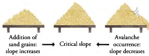
Figure 24.3. Self-organizing criticality (SOC): The sand pile model. Growing instability of a system (i.e., increased entropy due to addition of sand grains) will result in a critical period (or slope) where the system will spontaneously restructure itself (i.e., redistribution of sand pile); in other words, demonstrate the phenomenon of emergent and spontaneous self-organization.
